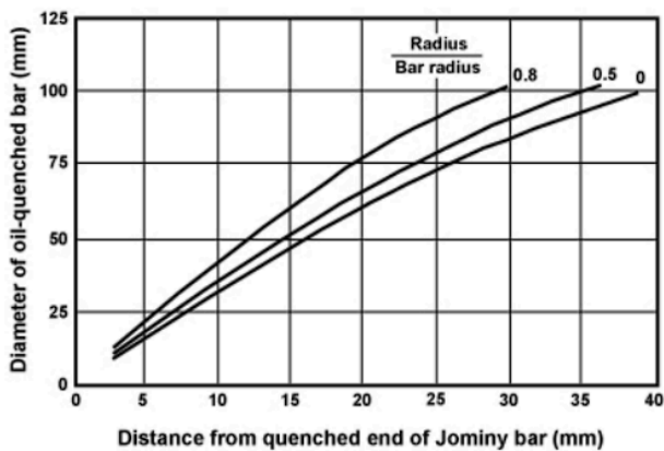
Jominy End-Quench Distance to Effective Diameter
